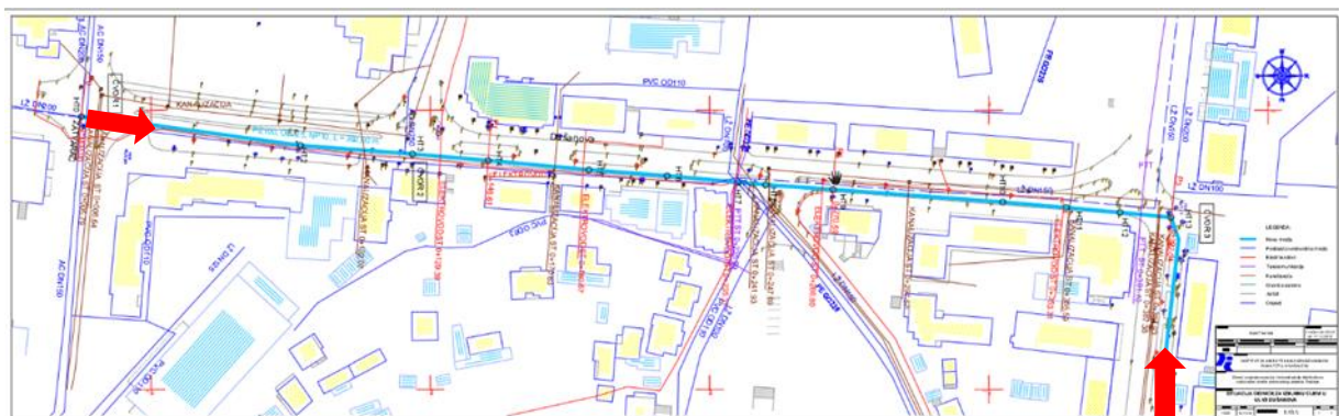
Figure 6. Situation of the pipe replacement section in Dušanova Street (Thick blue line – new pipeline)
