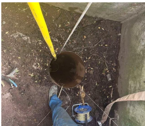
Figure 35. Performing pumping tests on the subject well and monitoring GWL on neighbouring wells
