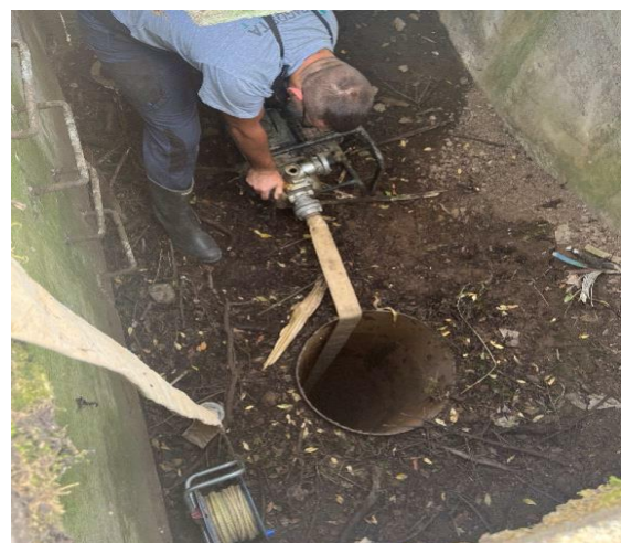
Figure 35. Performing pumping tests on the subject well and monitoring GWL on neighbouring wells
